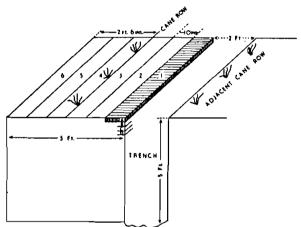
Fig. 15. Illustration of the digging procedure.
