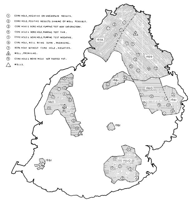
Fig. 11. Map of Mauritius showing areas surveyed by electrical resistivity (shaded). Sites of core holes, bore holes and wells are indicated.
